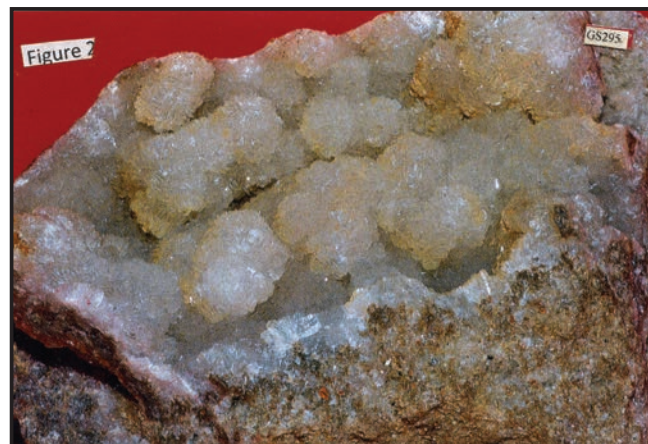
Figure 2. Closeup of hemimorphite crystals from the Mud Zone, Sterling Mine. Specimen dimensions: 9.5 × 7 × 2.5 cm (3.7 × 2.8 × 1 inches). Horizontal FOV is 8 cm (3.1 inches).
