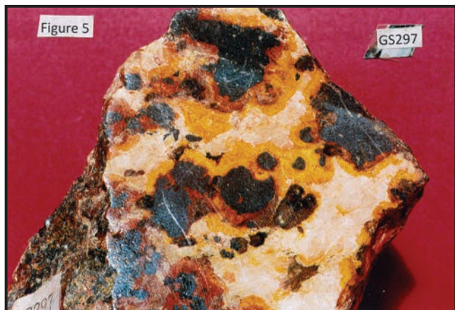
Figure 5. Orange zincite reaction rims around partly altered franklinite. North Ore Body, Sterling Mine. Specimen dimensions: 11.5 × 7 × 6 cm (4.5 × 2.8 × 2.4 inches). Vertical FOV is 4.8 cm (1.9 inches).
