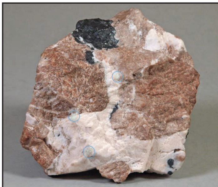
Figure 1. Coarse-grained willemite-franklinite-calcite ore from Sterling Hill, containing three grains of pale green genthelvite, the largest about 3 mm across. The genthelvite grains (circled), one just above the center of the specimen and two in the lower left quadrant, are inconspicuous in daylight but stand out brilliantly under LW ultraviolet light. Michael Isaacson specimen, 3.0 × 2.4 × 1.6 inches (7.5 × 6 × 4 cm). Earl R. Verbeek photo.
