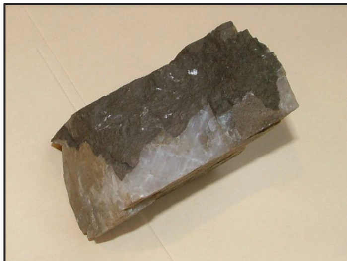
Figure 4. A fragment taken from a weathered block of lean franklinite-calcite ore, showing the dark, rough, weathered surface and relatively fresh calcite beneath.
