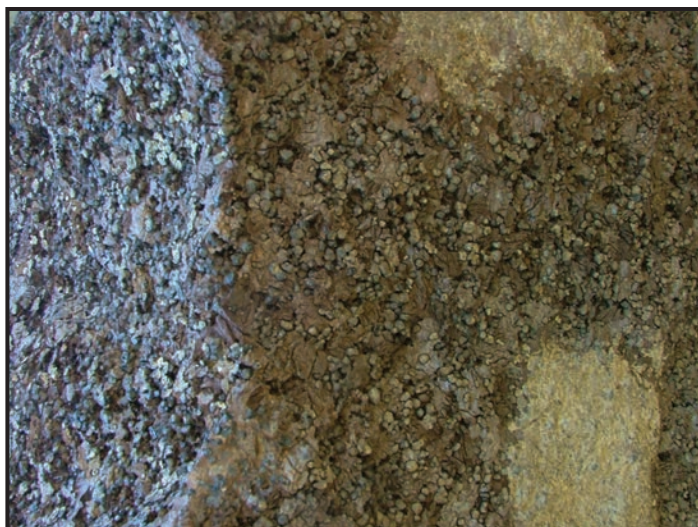
Figure 3. Rough surface of a block of franklinite-calcite zinc ore, showing franklinite grains standing in strong relief due to dissolution of the enclosing calcite. Franklinite grains freed by weathering have, in places, accumulated in deposits several inches thick at the base of long-exposed blocks of ore.
