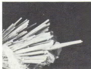
Figure 7. (third from top) Fibrous composite aggregate of hausmannite crystals. True width of horizontal field is 0.425 mm.
