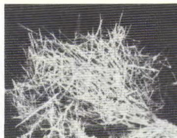
Figure 6. (second from top) Prismatic groutite crystals. True width of horizontal field is 3.0 mm.
