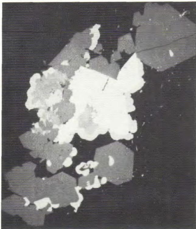
**Figure 1.** Backscattered-electron image of kentrolite (white), hetaerolite (gray), and calcite (dark gray). Magnification is 150x.
