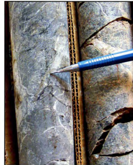
Figure 8. Close-up of thrust fault between Precambrian gneiss (top) and Paleozoic dolomite (bottom) in drill core from hole DR2. Fault plane in the core dips at an angle of about 60°, but the dip becomes much gentler to the east of the core hole. Pencil tip points to the fault contact.
