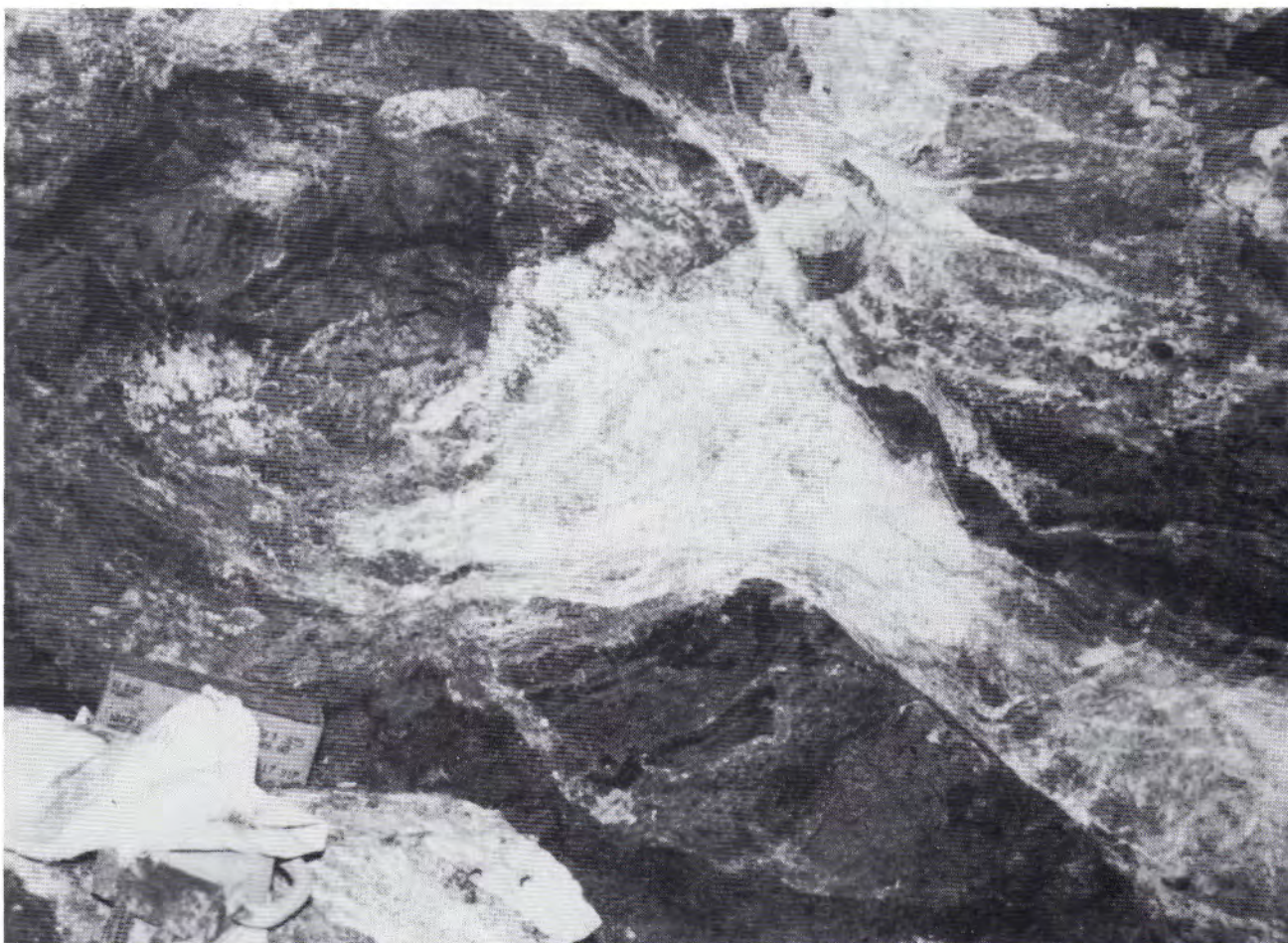
Figure 2a. West end of the pod of wollastonite-bearing rock, looking north, 740 crosscut, 700 level. Note contortion of wollastonite-bearing rock, and fingers of wollastonite-bearing rock extending into pyroxene calcsilicate rock. Field of view is about 0.7 m across; Steven Misiur photograph.
